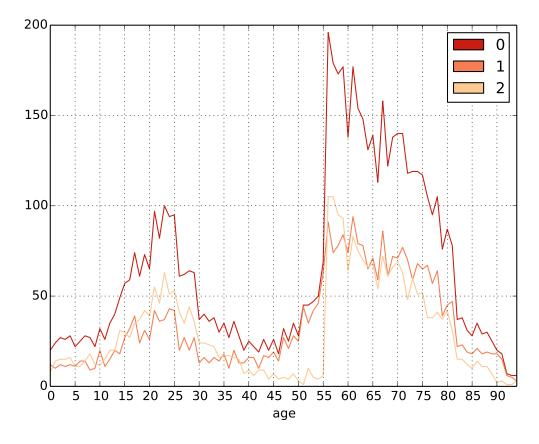
The third option is to pass (an expression returning) a two-dimensional array (plot (2d\_expr, ...)) in which case, there will be one line for each possible value of the first dimension and the second dimension will be plotted along the x axis. For example:
